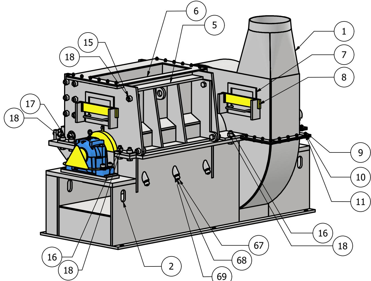
\*HOG SHOWN DOES NOT HAVE HYDRAULIC ADD-ONS. IF A HYDRAULIC REAR DOOR OPENER HAS BEEN INSTALLED, THE REAR DOOR WILL HAVE AN ADDITIONAL FLANGE FOR MOUNTING THE HYDRAULIC CYLINDER. THERE WILL ALSO BE A HYDRAULIC PUMP AND CONTROL VALVE BOX MOUNTED TO THE HOG HOUSING.
