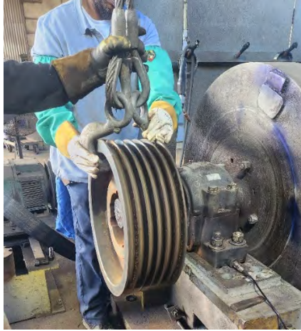
Figure 4.84: Lifting Outer Bushing Off Hog Shaft
