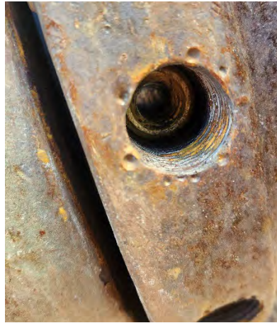
Figure 4.128: Top Half of Sheared Shear Pin
