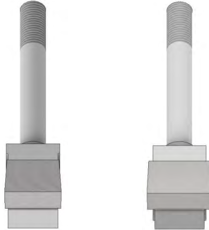
Figure 3.39: T3 Tooth – Standard Cut (Left) vs. Overlapping Cut (Right)
