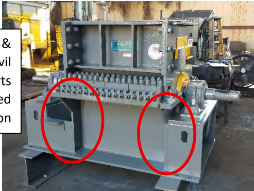
Figure 3.20: HD Anvil Supports (Left) vs. PM Anvil Supports (Right)
