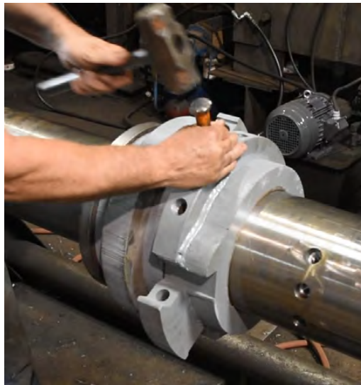
Figure 13: Driving Shear Pin into Position
