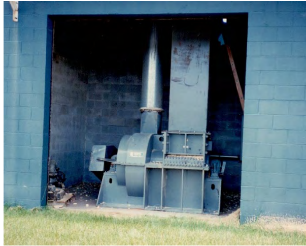
Figure 2.4: Hog Mounted Directly to Foundation
