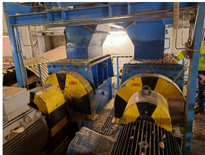
Figure 4.57: Redundancy Minimizes Downtime Following Hog Wreck
