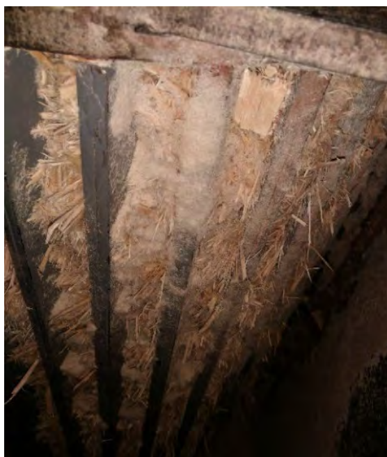
Figure 5.36: Screen Plugging from Incompatible Material
