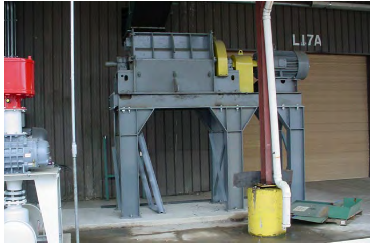
Figure 2.6: Hog Mounted on Sub-Base with Steel Column Legs
