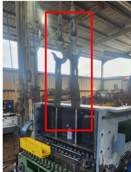
Figure 4.64: Lifting Device Secured to Front Door
