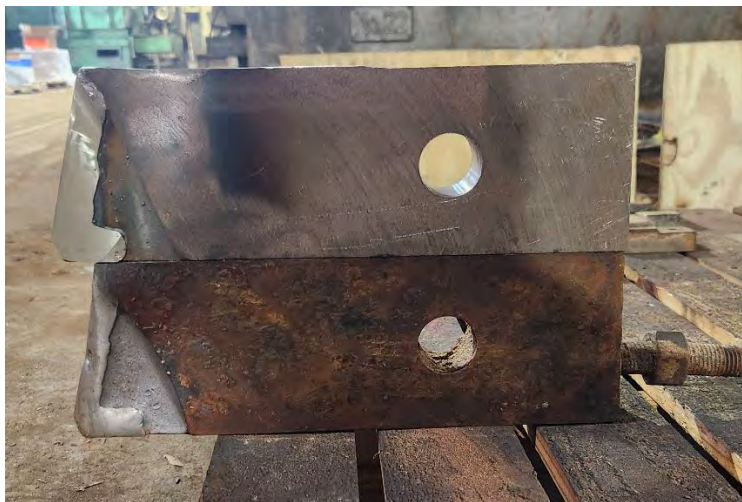
Figure 4.108: New vs Worn Large F Anvil
