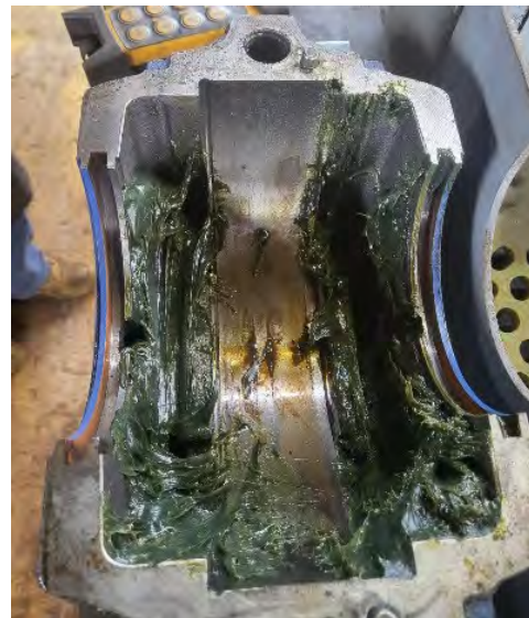
Figure 2.10: Bearing Unit and Housing Properly Packed with Grease
