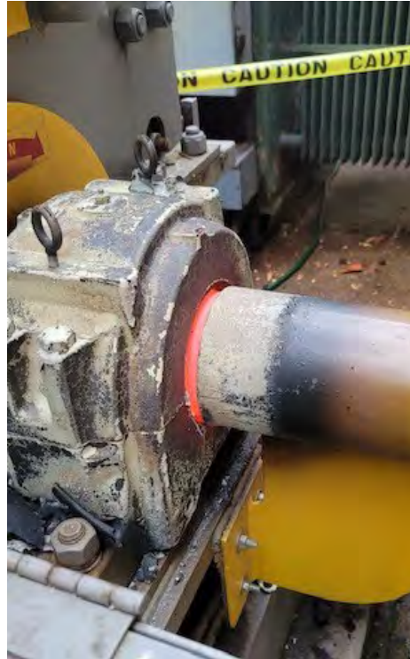
Figure 5.3: Overheated Bearing from Extended Use Without Lubrication
