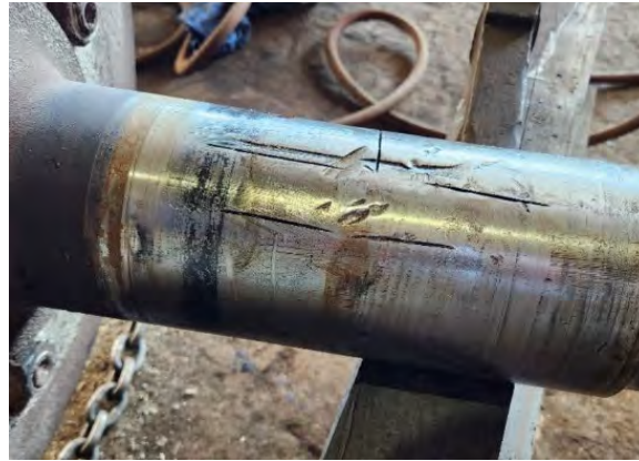
Figure 4.79: Gouged Shaft from Improper Component Removal
