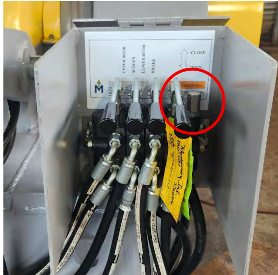
Figure 5.34: Hydraulic Relief Valve on Control Valve Block
