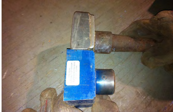
Figure 4.107: New VS Worn Tooth
