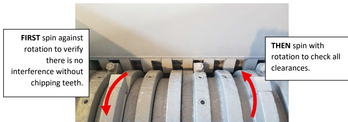
Figure 4.14: Verifying Clearance
