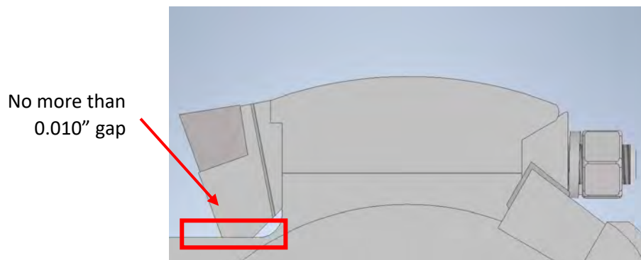
Figure 5.9: Gap on Tooth Seat
