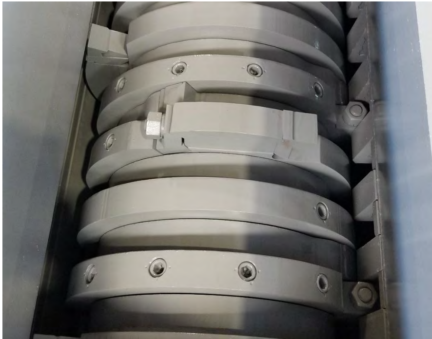
Figure 17: Dimples Around Every Setscrew
