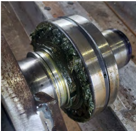
Figure 2.10: Bearing Unit and Housing Properly Packed with Grease
