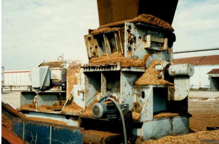
Figure 5.24: Chip Spillage through Unmaintained Hog
