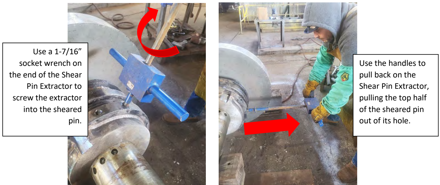
Figure 4.129: Shear Pin Extractor Operation
