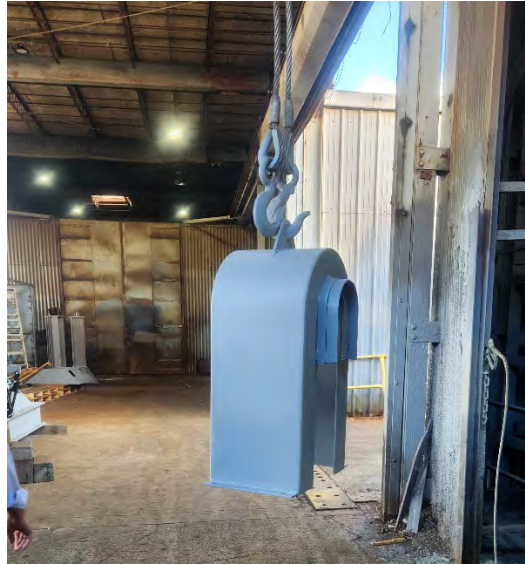
Figure 4.68: Proper Lifting of Direct Drive Motor Coupling Guard Cover
