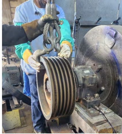
Figure 4.73: Lifting Outer Bushing Off Hog Shaft
