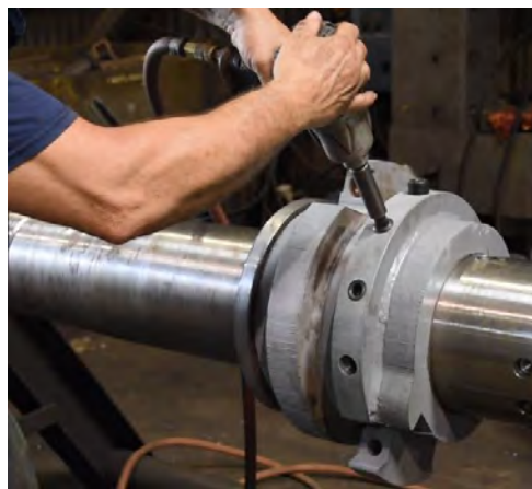
Figure 4.126: Fastening Set Screws
