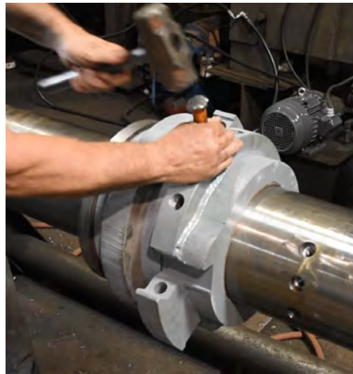
Figure 13: Driving Shear Pin into Position
