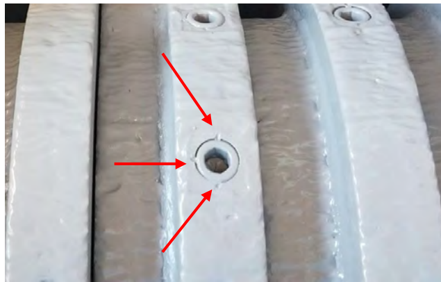
Figure 4.113: Locking Dimples on Setscrews
