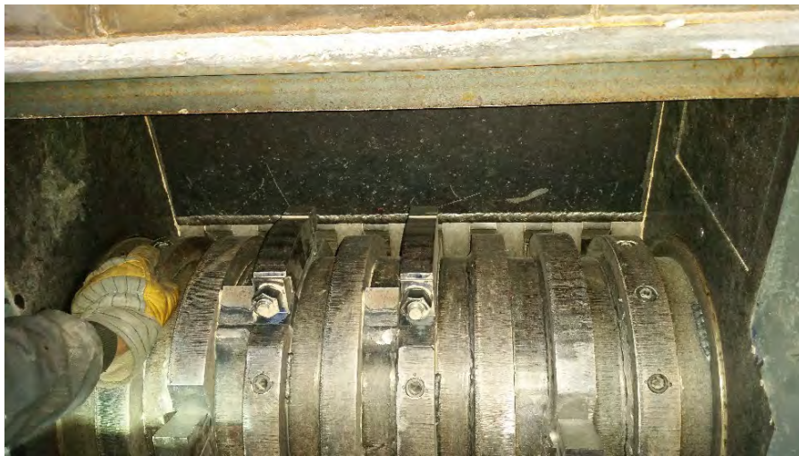
Figure 4.26: Turning Rotor by Hand to Ensure Clearances
