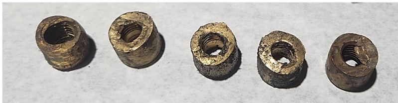
Figure 4.120: Pinched Shear Pins
