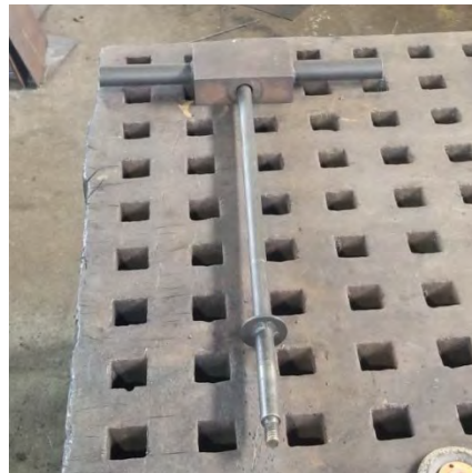
Figure 4.76: Shear Pin Extractor
