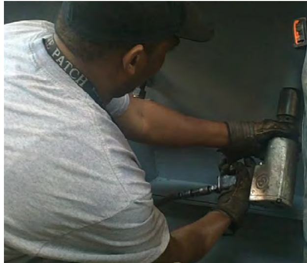
Figure 4.98: Removing Screen Hold Down Bolt Fasteners
