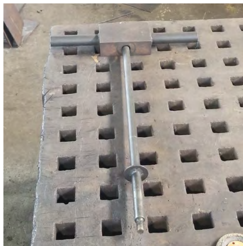
Figure 7: Shear Pin Extractor
