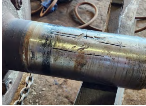
Figure 4.68: Gouged Shaft from Improper Component Removal
