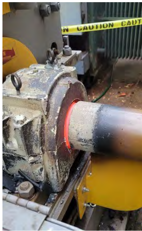
Figure 5.2: Overheated Bearing from Extended Use Without Lubrication
