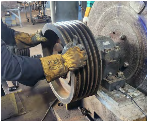
Figure 4.72: Jogging Loose from Taper
