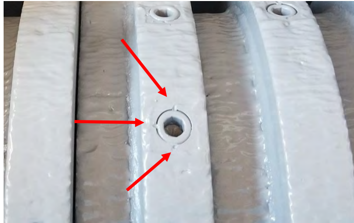
Figure 6: Locking Dimples on Setscrews
