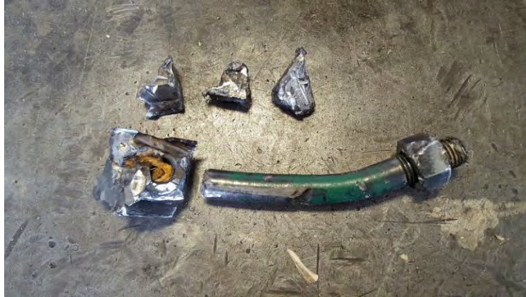
Figure 5.10: Mangled Tooth After Impact with Large Tramp Metal
