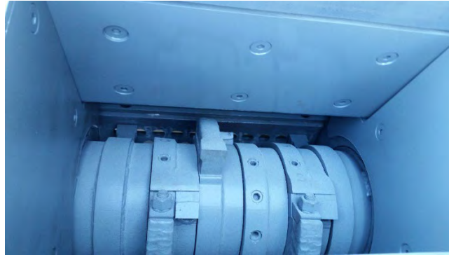
Figure 3.18: Rechipper Wear Plates
