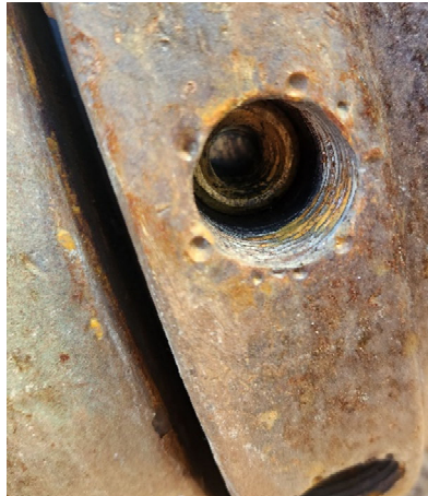
Figure 4.115: Top Half of Sheared Shear Pin
