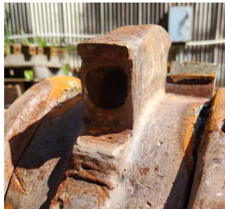
Figure 5.9: Egg-shaped Tooth Counterbore
