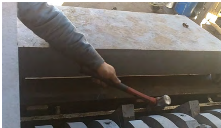
Figure 4.107: Driving Screen into Position
