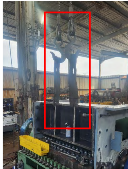
Figure 4.56: Lifting Device Secured to Front Door
