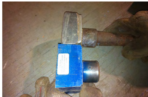
Figure 4.95: New VS Worn Tooth
