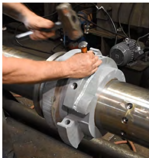
Figure 4.123: Driving Shear Pin into Position
