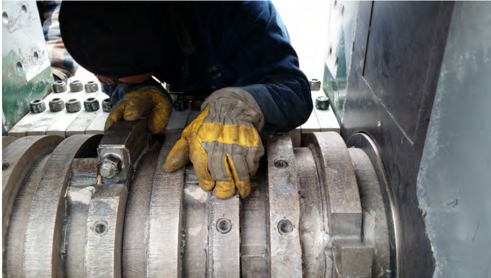
Figure 4.25: Verifying Tooth-Anvil Clearances
