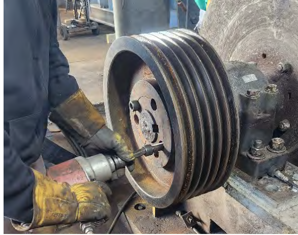
Figure 4.71: Tightening Screws into Back-Out Holes
