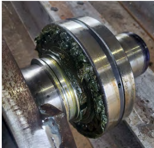
Figure 2.7: Bearing Unit and Housing Properly Packed with Grease
