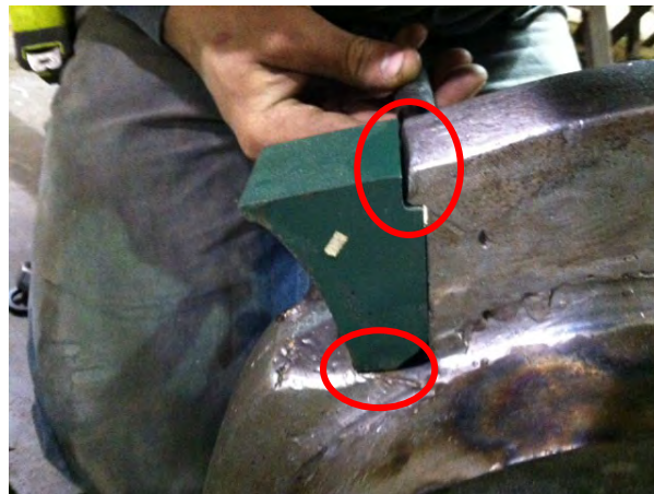
Figure 5.11: Gaps from Abrasion Wear
