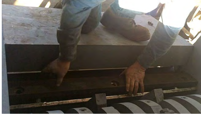
Figure 4.106: Reinstall Screen Clamping Bar
