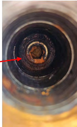
Figure 4.122: Removing Lower Half of Shear Pin
