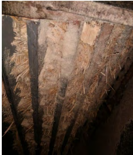
Figure 5.26: Screen Plugging from Incompatible Material
