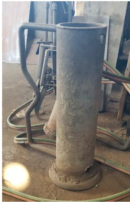
Figure 4.34: Bearing Removal Device
