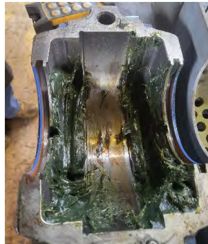
Figure 2.7: Bearing Unit and Housing Properly Packed with Grease
